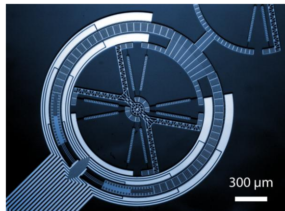
Figure 2: Micrograph of a micromotor fabricated in a single-crystal silicon, using a simple single-mask process, based on standard Silicon-On-Insulator technology.
