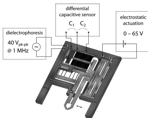
**Figure 1** Three-dimensional schematic of the MEMS nanotweezers fabricated with SOI technology.
