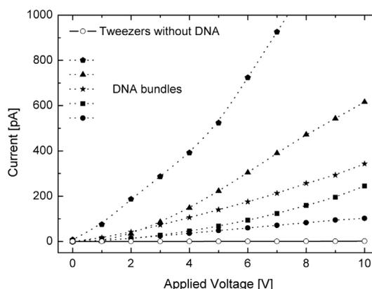
**Figure 4** Electrical characterization of DNA bundles with different diameters. Measurements done at room temperature (25°C), with ~50-60% humidity. The bundle diameters range from 100 nm to few μm.
