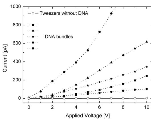
**Figure 4** Electrical characterization of DNA bundles with different diameters. Measurements done at room temperature ( $25^{\circ}\text{C}$ ), with ~50-60% humidity. The bundle diameters range from 100 nm to few  $\mu\text{m}$ .
