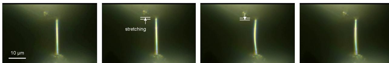
**Figure 5** Sequence showing the elongation of a DNA bundle by oscillating silicon nanotweezers. Movie taken at room condition under a Keyence VHX-500 Digital Microscope (× 5000 magnification).
