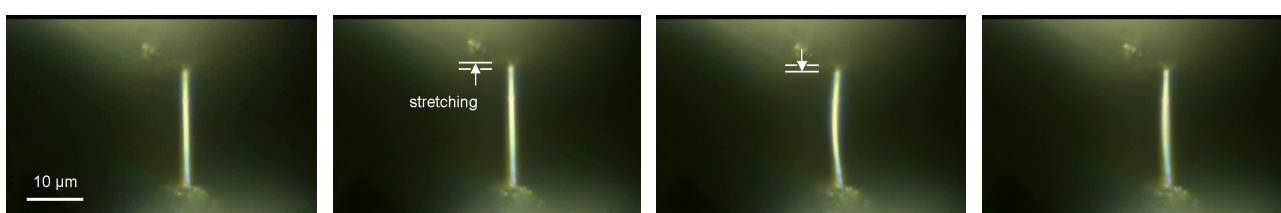
**Figure 5** Sequence showing the elongation of a DNA bundle by oscillating silicon nanotweezers. Movie taken at room condition under a Keyence VHX-500 Digital Microscope ( $\times 5000$  magnification).
