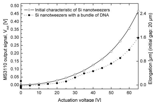
**Figure 3** Mechanical stretching of a bundle of DNA. A clear increase of the stiffness could be observed after the retrieval of a bundle of DNA.
