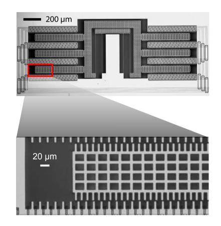
E. Sarajlic *et al.*, "Electrostatic 3-phase linear stepper motor fabricated by vertical trench isolation technology," *J. Micromech. Microeng.* **19** (7), No. 074001, 2009
