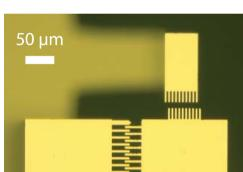
Video frame rate:  $f_{s} = 14.9763 \text{ Hz}$   $[f_{s} \approx 15 \text{ fps (tech. spec.)}]$ Oscillation frequency:  $f_{M} = \omega/2\pi = 2007 \text{ Hz}$ Aliased frequency:  $f_{alias} = |f_{M} - N \times f_{s}| = 0.1758 \text{ Hz}$ with N = 134
