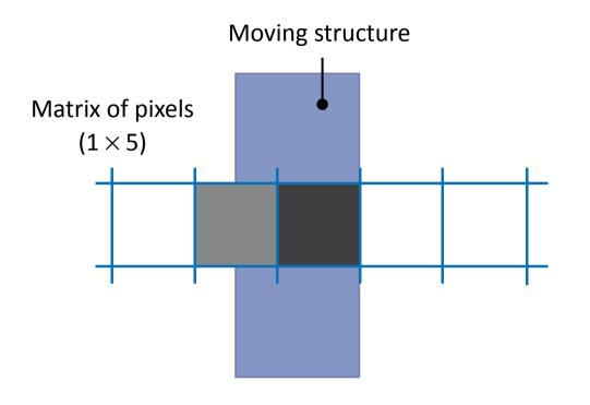
Subpixel resolution can simply be obtained by gray scale level interpolation.
